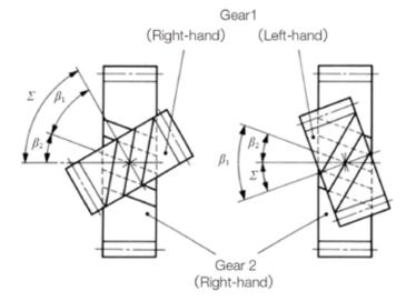
Figure 1: Screw gears of nonparallel and nonintersecting axes.
